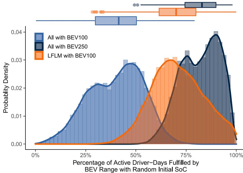
**Fig. 2.** Sensitivity of BEV suitability to initial State of Charge (SoC) based on stochastic simulation with 10,000 iterations. Initial SoC is uniformly distributed between 20 and 100%, and all other procedural details are the same as in Fig. 1. The average percentage of active days completed by BEV250 (BEV100) is 82% (40%). The simulation of specifically the LFLM driver cohort shows 71% of active days can be fulfilled with BEV100.
