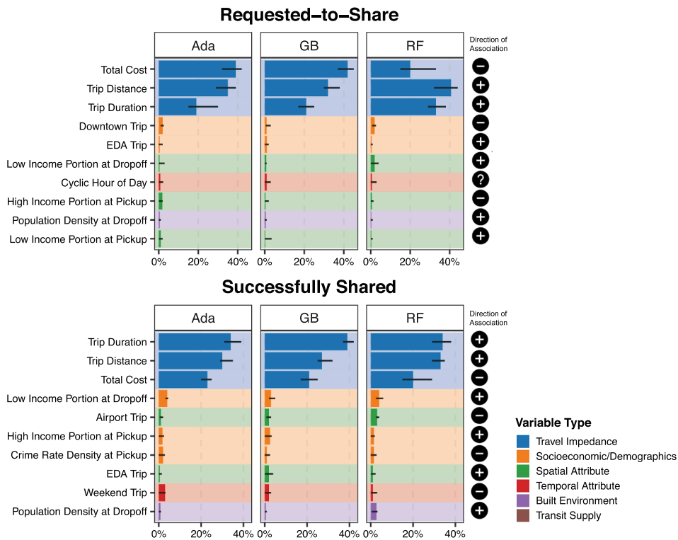
Fig. 6. Normalized relative predictive power of variables based on permutation feature importance with 5-fold cross-validation. Only top ten variables with the highest median predictive power are shown. The direction of association for each variable is determined using partial dependence analysis.
